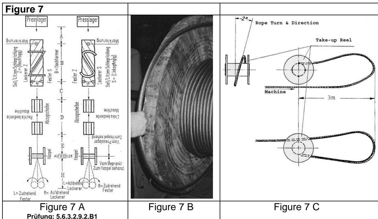
**Turns in strands** depending on Type of lay and rope/strand construction.
