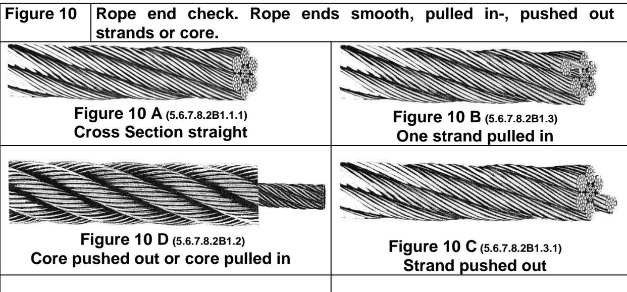
**7. Testing of ropes and testing of rope quality. Final rope inspection.**
