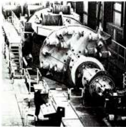
Fig. 6: Adequate bobbin capacity permits the production of ropes in one length for multiple hoisting rope installations
